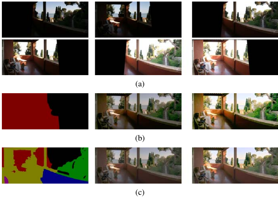
Figure 10.17 HDR merging with large amounts of motion (Eden, Uyttendaele, and Szeliski 2006) © 2006 IEEE: (a) registered bracketed input images; (b) results after the first pass of image selection: reference labels, image, and tone-mapped image; (c) results after the second pass of image selection: final labels, compressed HDR image, and tone-mapped image
