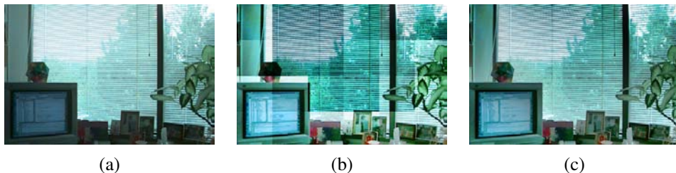
Figure 3.8 Locally adaptive histogram equalization: (a) original image; (b) block histogram equalization; (c) full locally adaptive equalization.
