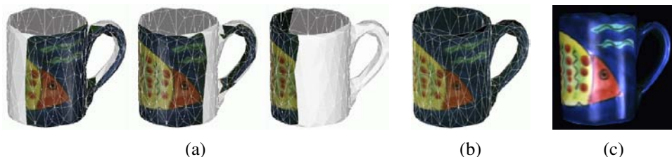
Figure 12.22 Estimating the diffuse albedo and reflectance parameters for a scanned 3D model (Sato, Wheeler, and Ikeuchi 1997) © 1997 ACM: (a) set of input images projected onto the model; (b) the complete diffuse reflection (albedo) model; (c) rendering from the reflectance model including the specular component.
