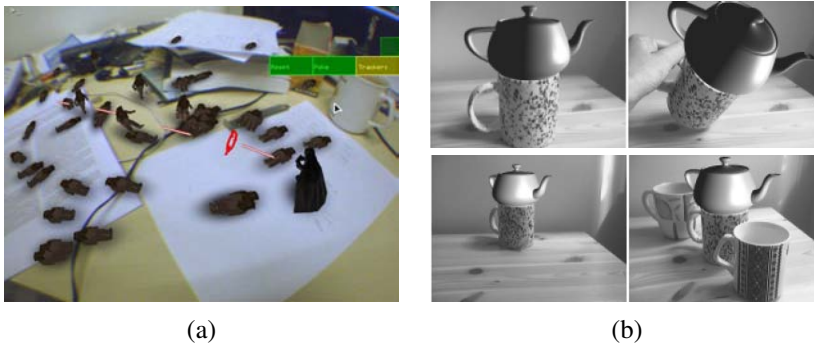
Figure 7.10 3D augmented reality: (a) Darth Vader and a horde of Ewoks battle it out on a table-top recovered using real-time, keyframe-based structure from motion (Klein and Murray 2007) © 2007 IEEE; (b) a virtual teapot is fixed to the top of a real-world coffee cup, whose pose is re-recognized at each time frame (Gordon and Lowe 2006) © 2007 Springer.
