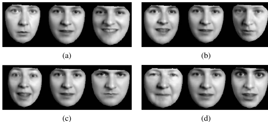
Figure 14.22 Principal modes of variation in active appearance models (Cootes, Edwards, and Taylor 2001) © 2001 IEEE. The four images show the effects of simultaneously changing the first four modes of variation in both shape and texture by \pm\sigma from the mean. You can clearly see how the shape of the face and the shading are simultaneously affected.
